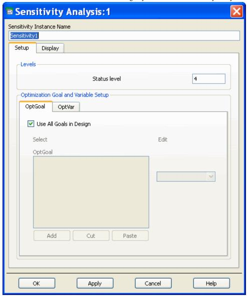
Sensitivity analysis comprises a single-point or infinitesimal sensitivity analysis of a design variable. For circuit design, it involves taking partial derivatives of the response with respect to a design variable of interest. It is thought that these numbers can help pinpoint variables that contribute disproportionately to performance variance.
